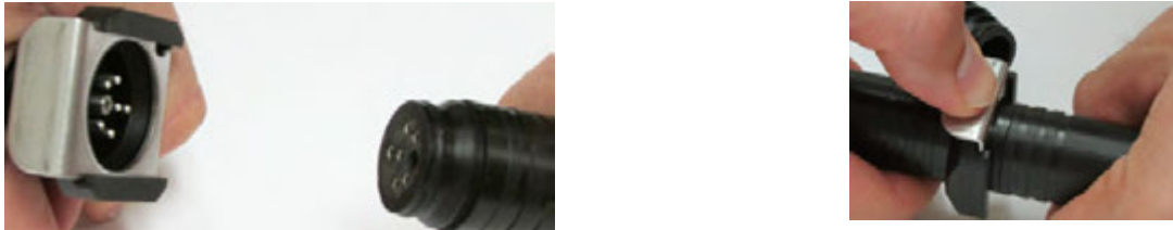
Figure 4-13 How to connect a TIENet receptacle to the Signature Portable
