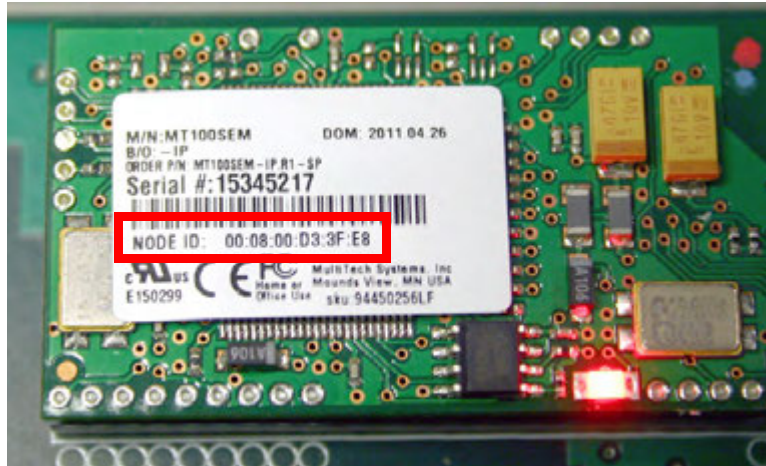
Figure 5-32 Locating the NODE ID (MAC address) on the ethernet modem
