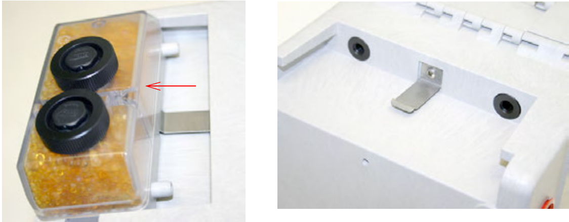
Figure 5-13 Removing the external desiccant cartridge
