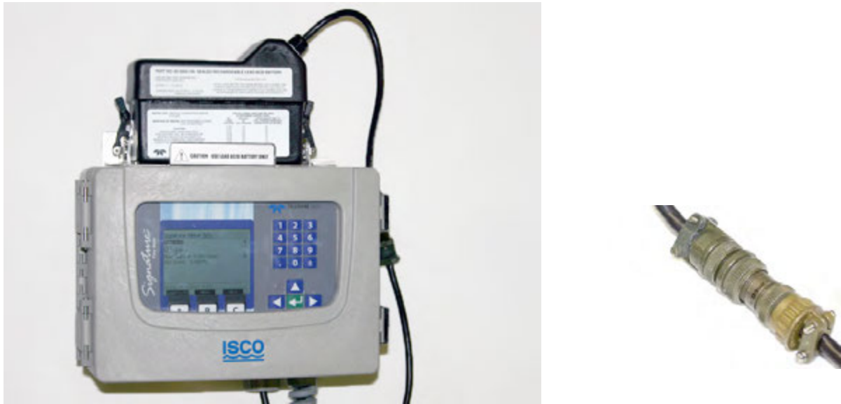
Figure 5-8 Backup battery, installed
